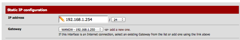
FIGURE II.4 – Menu Interfaces : configuration de l’interface WAN
