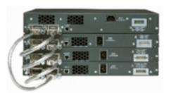
Stackable switches, connected by a special cable, effectively operate as one large switch.
